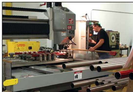
Haas Gantry Router Machine
