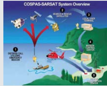
Beacons with 406Mhz, 121Mhz and GPS technologies signal for rescue from far away
